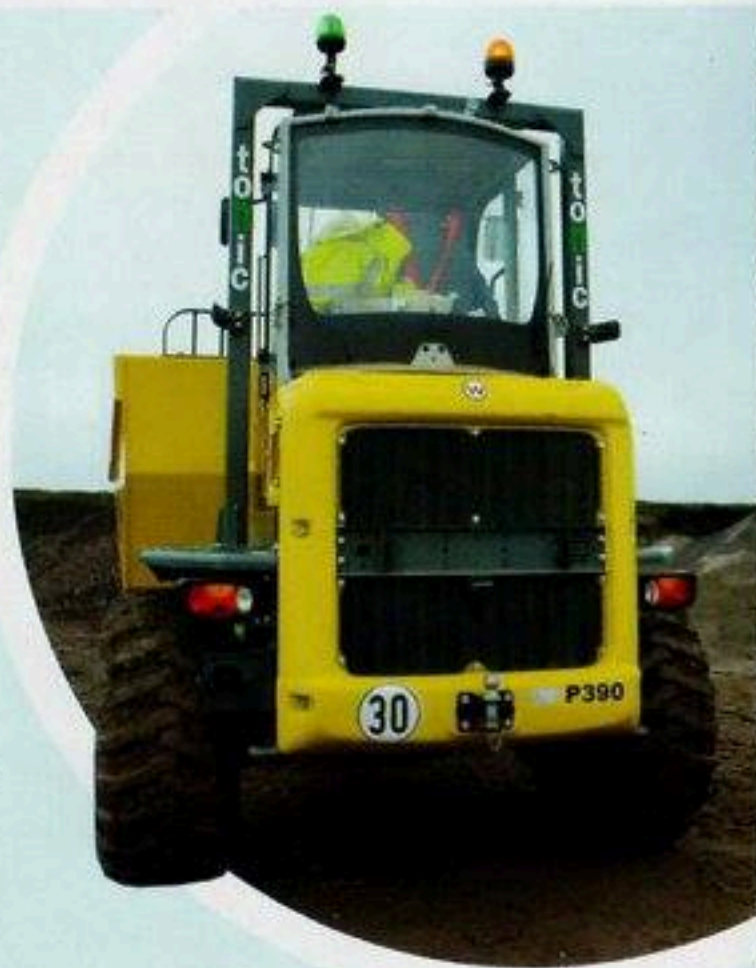
Above, below and below far left: A redesigned skip to provide a lower front lip plus larger tyres than standard all help to improve visibility and stability.
