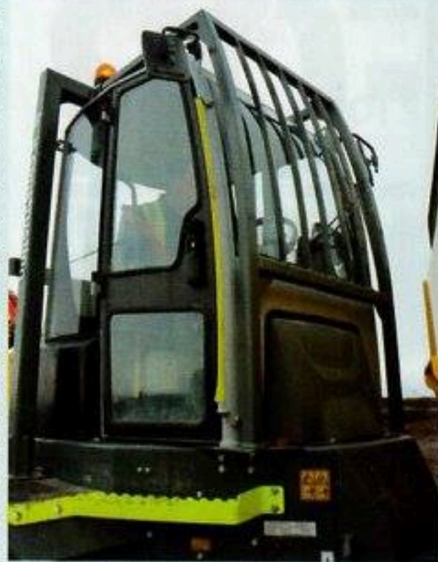
The additional cab guarding is to withstand the impact of an excavator's bucket during loading.
